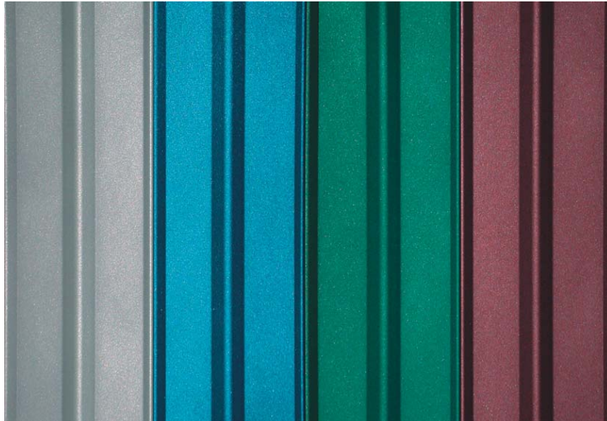
Figure 40: Different colours are available for efficient absorber layers (picture source: AEE INTEC).
